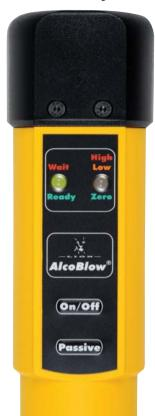
**On/Off switch** - press and release once to switch on, then once again to switch off.
